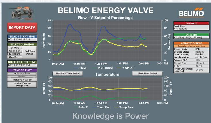
The software monitors and can trend all sensed or calculated values for up to 13 months. These values include water flow, return and supply water temperature, power, energy, or media density and more.
